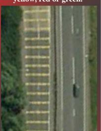
HSR provides a visible, audible and a physical 'thump' warning to the driver through the vehicle tires that they need to slow down, it is made reflective using glass beads to maximise visibility at night and contains calcined bauxite for high skid resistance.
